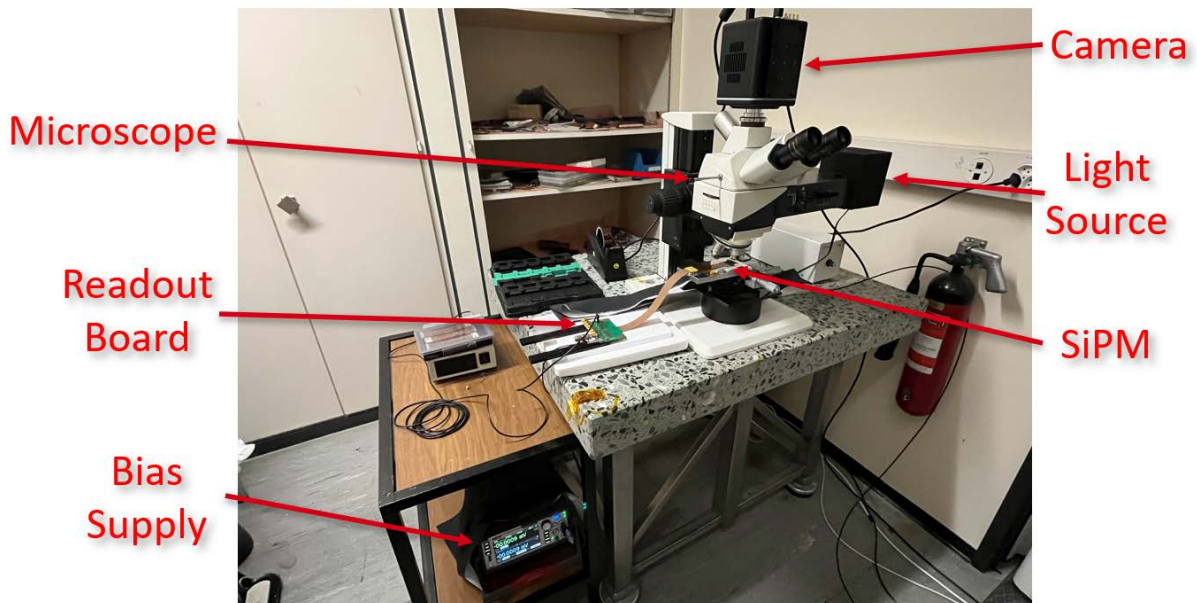
Figure 13: The emission-microscopy bench used in this project. The cooled qCMOS camera is mounted on the microscope, beneath which the SiPM is held flat by a vacuum chuck; the bias supply is connected to the SiPM through a readout board, while a halogen lamp provides the illumination used only for the short reference exposure.
