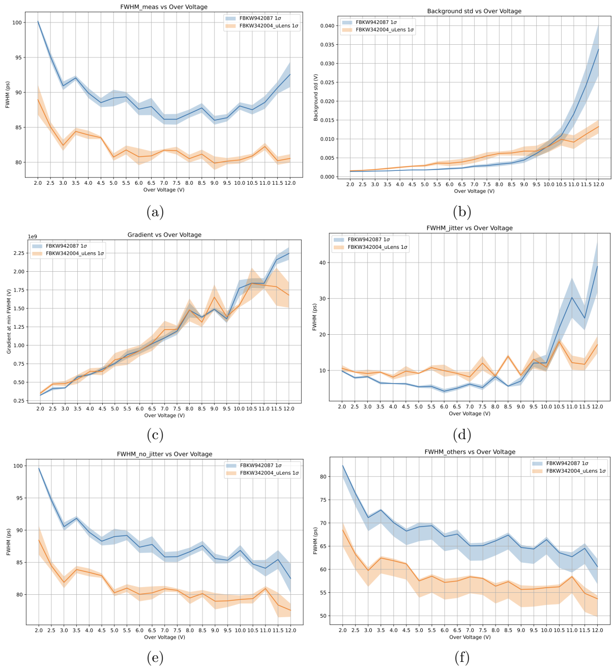
Figure 22: Average results across different channels of FBK942087 and FBK342004 \mu Lens. While both devices reach \text{FWHM}_{\text{meas}} saturation beyond 7V, FBK342004 \mu Lens consistently performs better by about 5 ps across the OV range. The microlens design contributes to reduced intrinsic timing error and improved SPTR.
