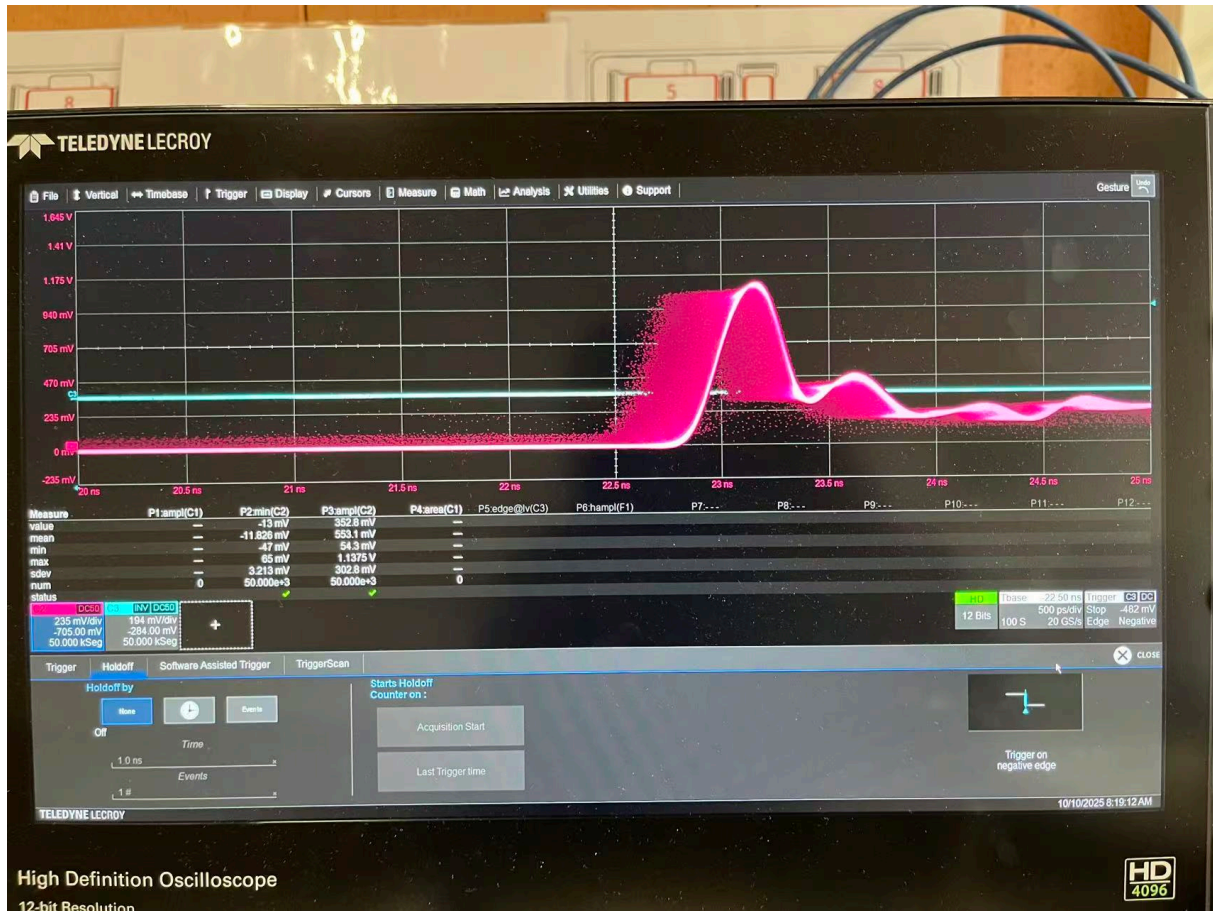
Figure 10: Oscilloscope used for SiPM waveform acquisition. The laser trigger serves as the time reference.
